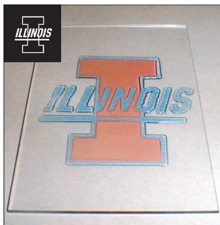
Figure 7. Multicolored polymer structures produced using complementary photomasks and different colored photoresists.
